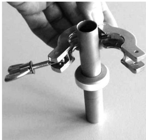
Fig. 61: Attaching the clamping ring
