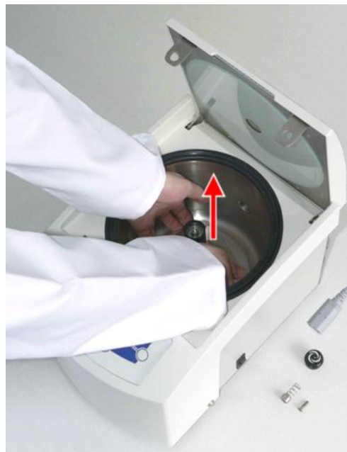
Fig. 43: Removing the rotor shaft
