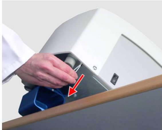
Fig. 36: Unlocking the lid locks
