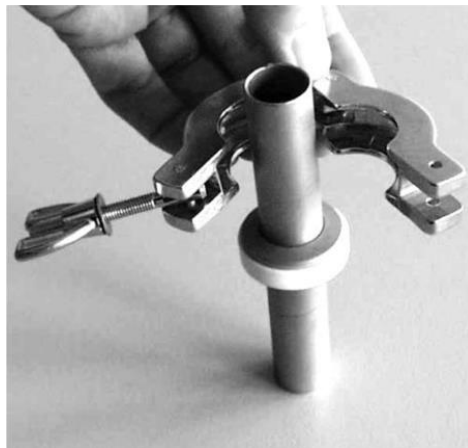
Fig. 39: Attaching the clamping ring
