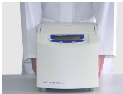
Fig. 7: Lifting the RVC
