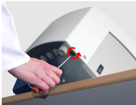
Fig. 34: Loosening of the plastic screw
