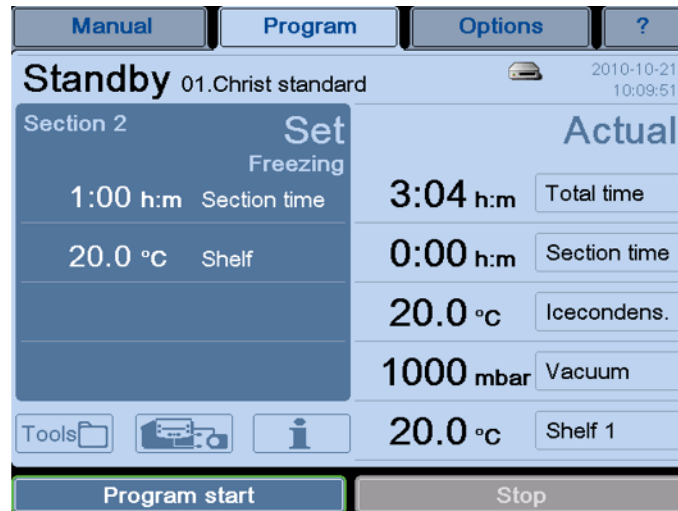
Fig. 68: The freeze-drying process can be started with the aid of the button "Program start".
