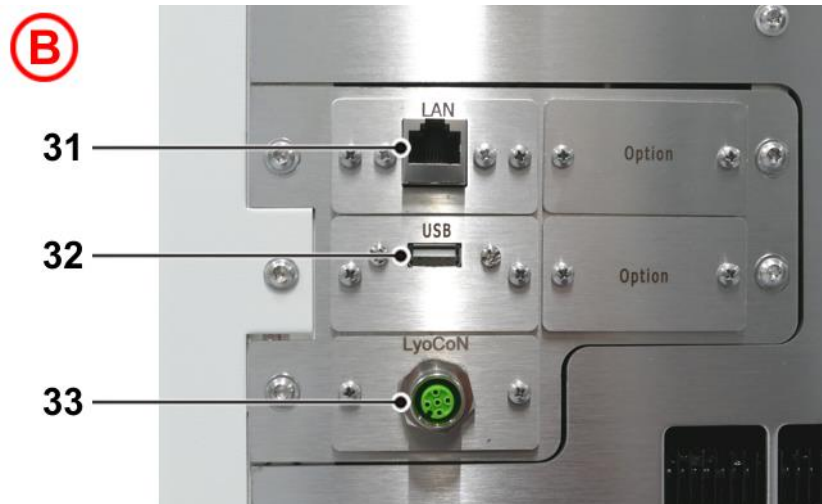
Fig. 6: Detailed view B – Connections on the rear side of the freeze dryer
