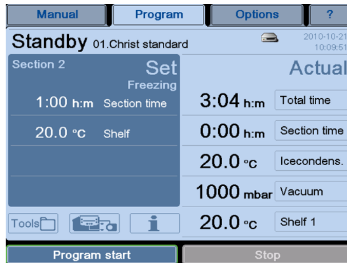
Fig. 68: The freeze-drying process can be started with the aid of the button "Program start".
