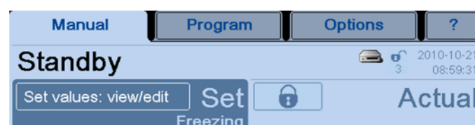
Fig. 44: Countdown of the password timer and the button with the lock symbol
