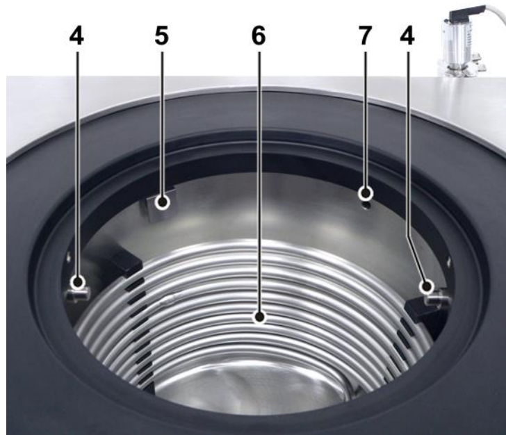
Fig. 3: Ice condenser chamber
