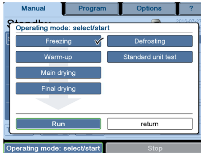
Fig. 29: Dialog box "Operating mode: select/start" (The version of the dialog box that is displayed depends on the equipment of the freeze-dryer.)
