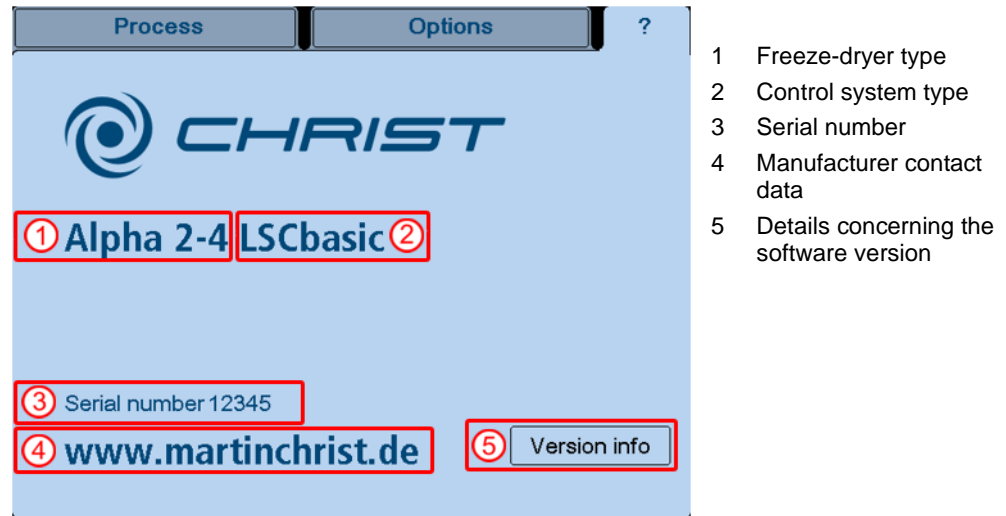
Fig. 48: Freeze-dryer system information (example)
