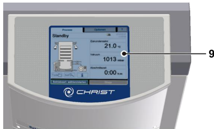
Fig. 4: User interface with touchpanel
