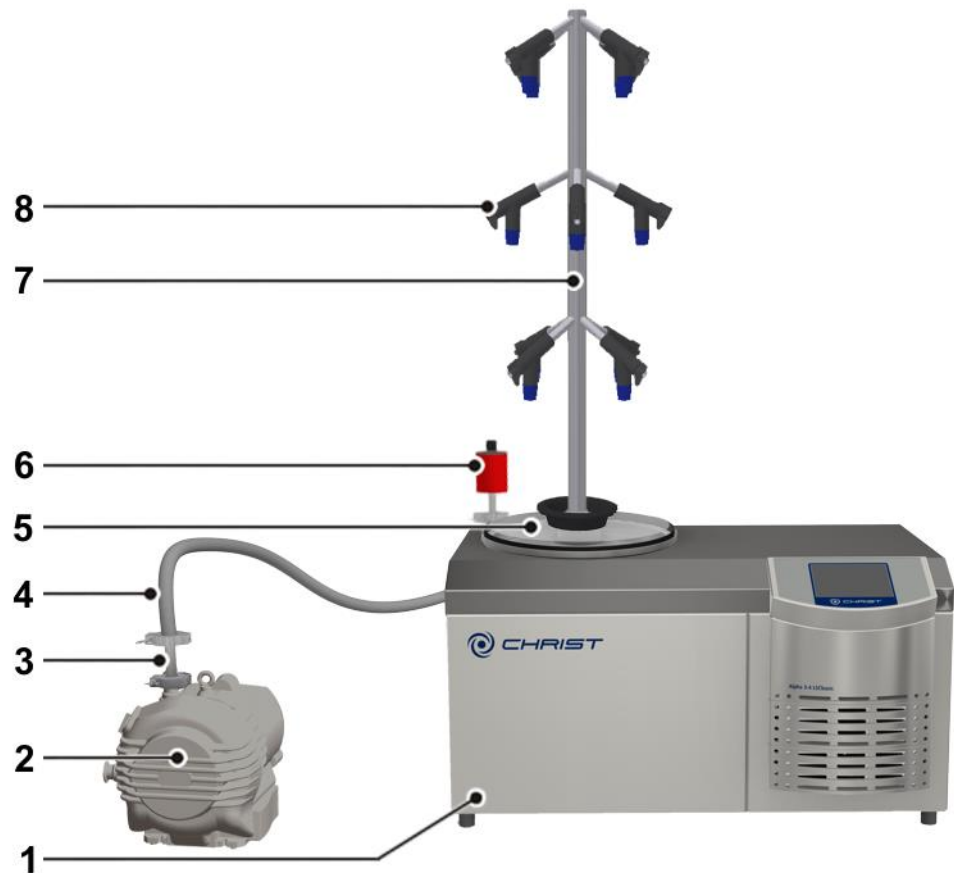
Fig. 19: Freeze-dryer Alpha 3-4 LSCbasic with solvent package flask and vacuum pump Pfeiffer Hiscroll 12 Atex or Edwards nXDS 10iC, part no. 102516 or 102486
