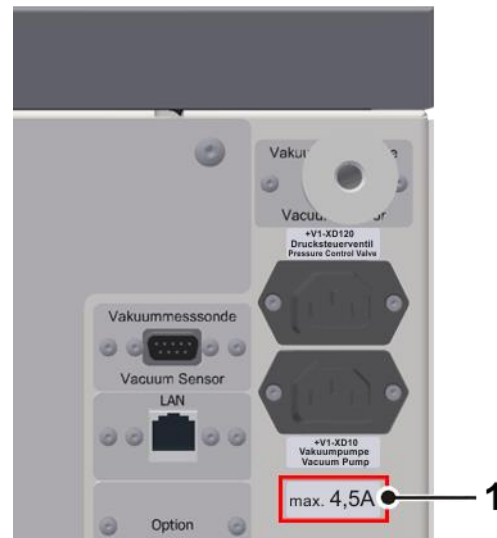
Fig. 12: Indication of the maximum current for the vacuum pump (example)
