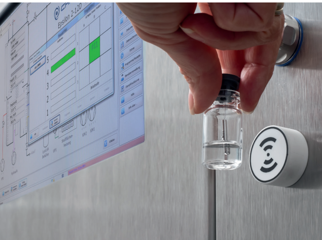
Automatic identification by RFID and integration in LPCplus
